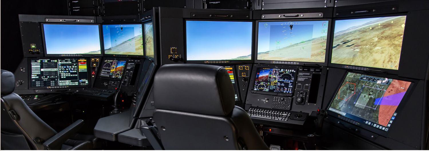
The GA-ASI Certifiable Ground Control Station contains parts previously made with laminated composites that are now 3D printed.
